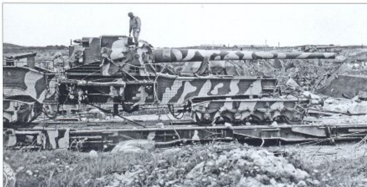
The army preferred heavy railroad guns over massive fixed guns for long-range firepower. This is a Krupp 203mm K(E) of battery EB.685 stationed near Auderville-Laye in the Cherbourg sector shortly after its capture in June 1944. (NARA)
