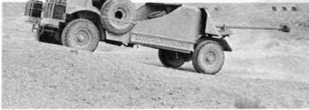
Trials of the Legion's prototype anti-tank vehicle constructed from a Ford-Canadian three-ton truck. December 1953
