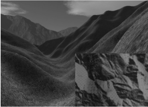
Figure 13.7. A camera is placed above the player from a bird's eye view and renders the scene into an off-screen texture. When we draw the scene from the player's eye to the back buffer, we map the texture onto a quad in the bottom-right corner of the screen to display the radar map.
