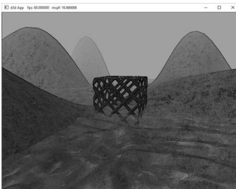
Figure 13.15. Multiplying the original image by the inverse of the edge detection image to produce a stylized look where edge look like black pen strokes.
