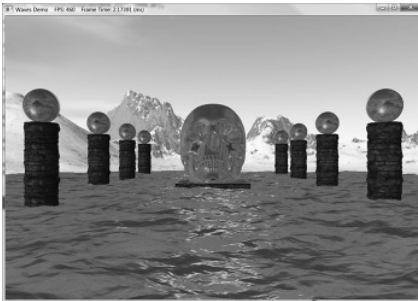
Figure 19.8. Ocean waves modeled with heightmaps, normal maps, and environment mapping.
