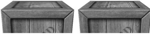
Figure 9.9. The top face of the crate is nearly orthogonal to the view window. (Left) Using linear filtering the top of the crate is badly blurred. (Right) Anisotropic filtering does a better job at rendering the top face of the crate from this angle.
