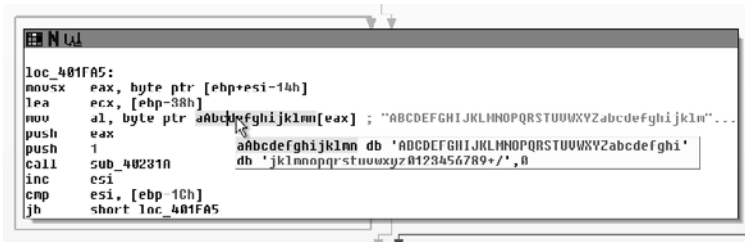
Figure 12-3: Following the cross-reference to the alphabet leads you to the base64 algorithm.
