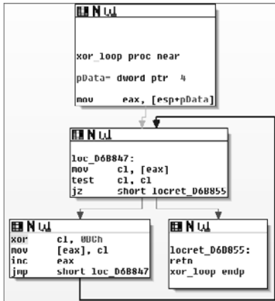
Figure 12-1: A function that performs single-byte XOR
