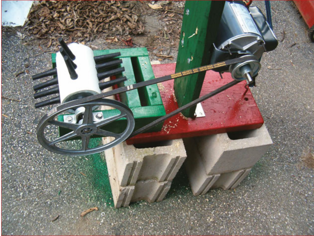
⤷ Plucker with belt and tensioner installed.
