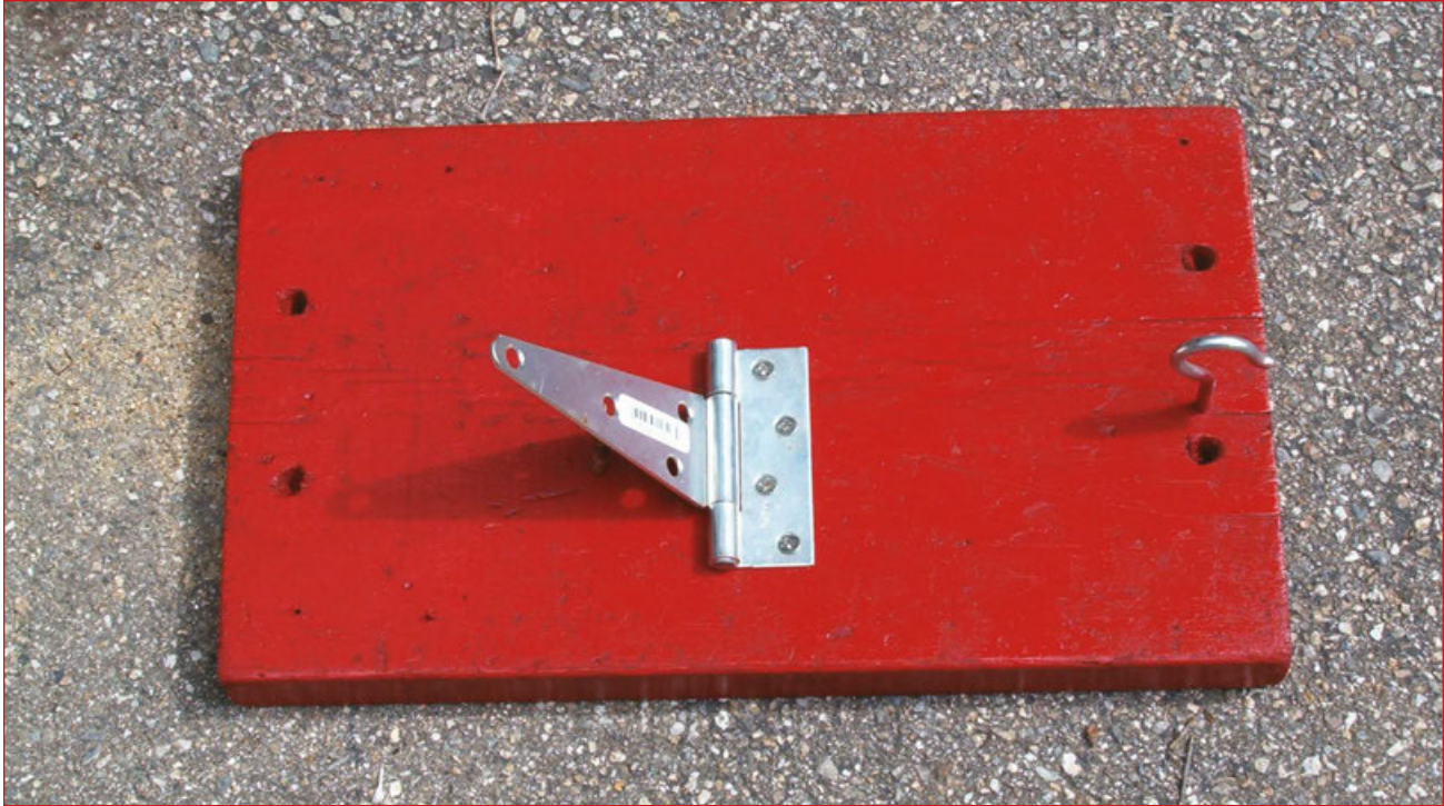
☞ The large board with hinge and hook installed.
