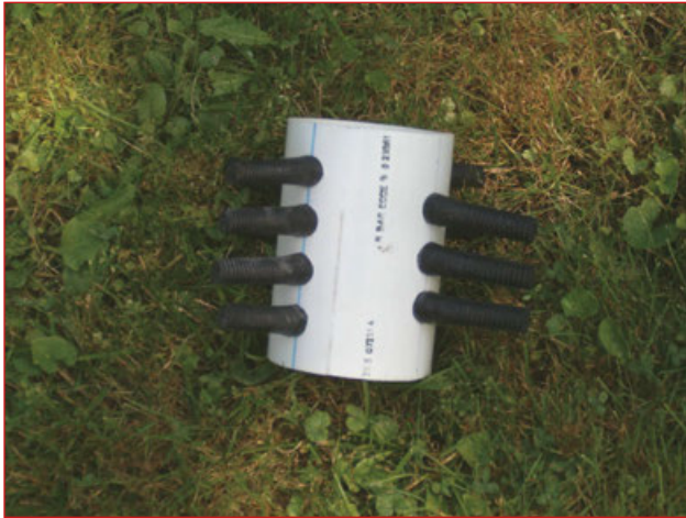
☞ Plucker drum with fingers installed.
