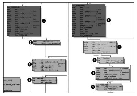
Figure 22-2: PatchDiff2 graphical function comparison
