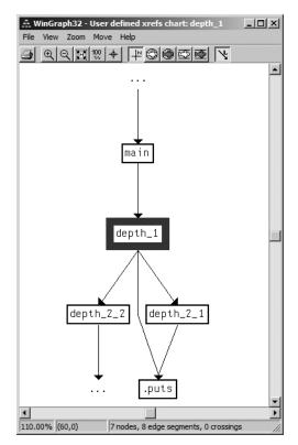
Figure 9-12: User xref graph for function depth\_1
