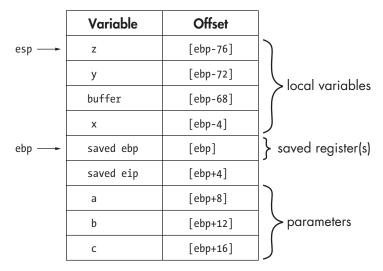
Figure 6-4: An EBP-based stack frame
