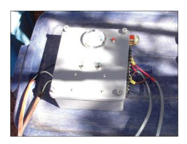
solar panel. The wires on the right side are going to the battery bank and dummy load. I cut up an old heavy-duty 100' extension cord to make cables to connect wind turbine and solar panel to the charge controller. The cable to the wind turbine is about 75 feet long and the cable to the solar panel is about 25 feet long. The battery bank I am currently using consists of eleven sealed lead-acid 12V batteries of 8 Amp-Hour capacity connected in parallel. That
