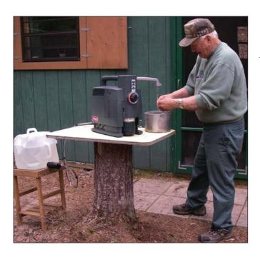
Coleman's propane-heated "Hot Water On Demand" unit is a very handy backup when utilities stop working, and there's even a shower attachment for personal hygiene and decontamination.
