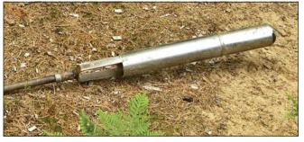
A pilot hole for the well point is drilled using a steel handauger that screws into the earth while jamming loosened soil into its hollow body, and increasing the depth of a neat round hole 10 inches each time it is pulled up to be emptied.
