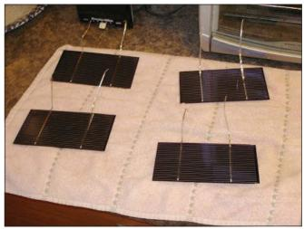
sides or they will warp when exposed to moisture. Warping could damage the solar cells that will be glued to them.
