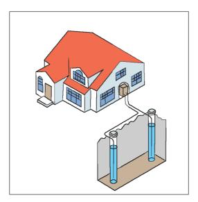
An open-loop heat pump system.
