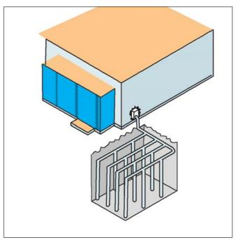
A vertical closed-loop heat pump system.
