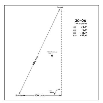
In this example, shooting at a target well above the shooter, the trajectory drop of the bullet will not be based on the actual bullet flight distance of 400 yards, but rather on 100 yards.
