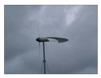
Wind turbine. The propeller is turned to face the wind. As it spins, it turns the generator of the turbine to create electricity.
