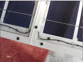
Step 9: Install the Half Panels in the Box
