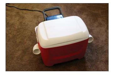
Is your refrigerator sucking up so much juice you can't run the AC? The improvised AC unit seen here uses one tenth the power your window AC does, and consists of a cooler with a couple of PVC elbows to direct the airflow. A fan on low speed blows air through a hole and across frozen plastic water bottles stacked inside the cooler.
