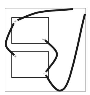
Batteries or solar panels wired in parallel. The voltage stays the same. The amps are added. These two 12V, 120-amp batteries wired in parallel produce 12 volts at 240 amps. Note that in parallel systems, the main cables must come from opposite corners to ensure that batteries are charged and discharged equally.
