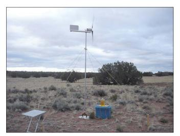
only slightly increase as the wind speed increases. More wind means more current into the battery which means more load on the generator. So the system is pretty much self-governing. I saw no signs of over-revving. Of course, in stormforce winds, all bets are off. Switching the controller to dump power
