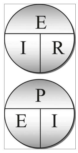
Use the circles to help remember the formulas for Ohm's Law (I = E/R, E = IR, R = E/I) and for power (E = P/I, P = EI, I = E/P).
