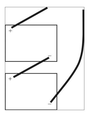
Power sources (batteries and solar panels) wired in series. The amperage stays the same, but the voltages are added. These two 12V, 120-amp batteries wired in series produce 24V at 120 amps.
