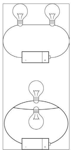
Top, a series circuit. The current flows through the components one after another. If one component stops working and breaks the circuit, no current flows. It's why an entire string of cheap Christmas lights stops working when a single bulb burns out. Bottom, a parallel circuit has more than one path for the current. If a component in one path stops working and breaks the circuit, current continues to flow through the other path.
