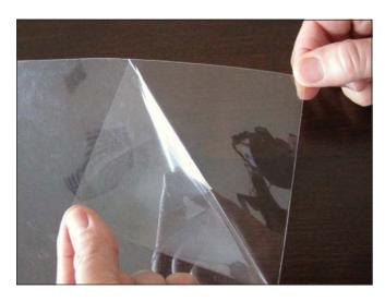
This photo is of laminate window reinforcement. Peel the backing off to expose the dry glue and apply to the window. Different thicknesses or multiple layers can be applied according to the threat (ballistic, explosive, high wind). The 0.009-inch and 0.011-inch thicknesses are the most commonly applied to residences and small businesses. The 0.003, 0.005, 0.006, 0.007, 0.014, and 0.020 are also available.
