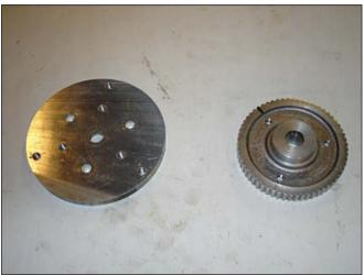
workshop, I found a toothed pulley that fit on the motor shaft, but was a little too small in diameter to bolt the blades onto. I also found a scrap disk of aluminum 5 inches in diameter and 1/4" thick that I could bolt the blades onto, but wouldn't attach to the motor shaft. The simple solution of course was to bolt these two pieces together to make the hub. Much drilling, tapping, and bolting later, I had a hub.
