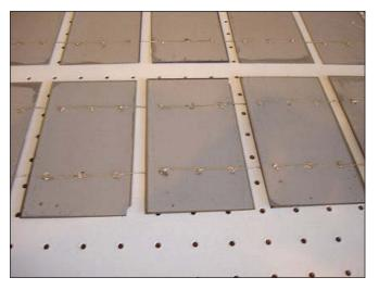
teasing the cells apart once the wax melts. Try not to pull too hard on the metal tabs or they may rip off. I found that out the hard way while trying to separate the cells. Good thing I bought extras.
