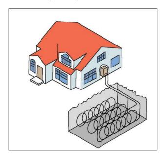
A horizontal closed-loop heat pump system.
