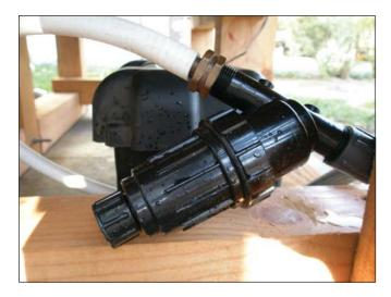
the Watersaver attachment for the  $3 \times 4$  downspout pipe works perfectly. In order to enable adequate water flow to the barrel, I adapted the Watersaver attachment by drilling out the side and adding a flange for a 1" PVC fitting. I sealed this by using
