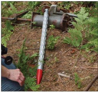
Essentially a stout hollow nail with screened intake ports, the typical 6well point provides access to subterranean water at depths to and exceeding 50 feet.
