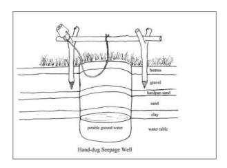
A seepage well is simply a hole dug straight down to the water table.
