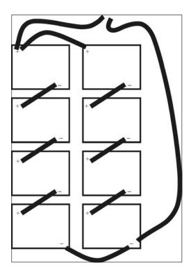
To increase both amperage and voltage, batteries or solar panels can be configured with strings of series batteries wired in parallel. This shows a 48V, 240-amp system made with 12V, 120-amp batteries.
