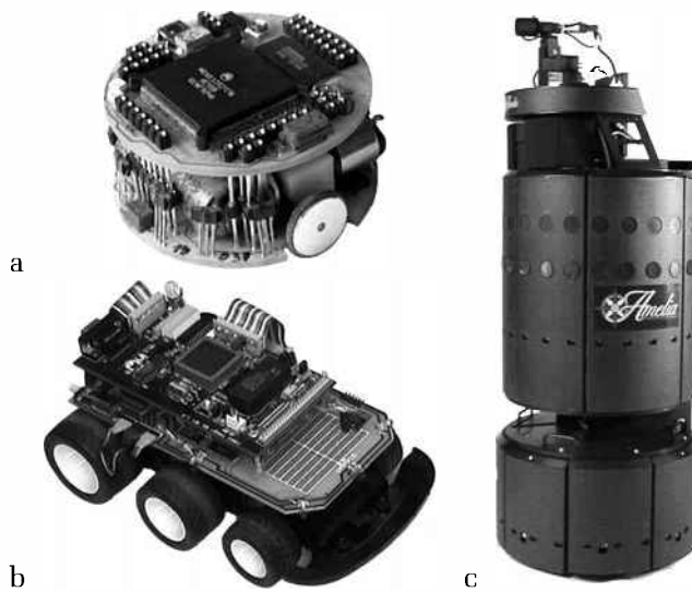
Figure 5.8 Different types of robots: (a) Khepera, (b) Didabot, (c) B21 from Real-World Interface. The Khepera robot is a widely used robot platform in the field of autonomous agents. It is especially convenient because of its small size. Khepera can be used by people who have only a superficial knowledge of robots. The Didabot is similar to the Khepera robot in basic functionality, but it is bigger, which makes it easier for the designer to add his or her own sensors. It can be built by students under supervision in a few days. B21 is, in a sense, the Rolls Royce of mobile robots. It comes equipped with, among many other things, sensory systems, including a stereo vision system. There are considerable differences in cost between the different platforms.
