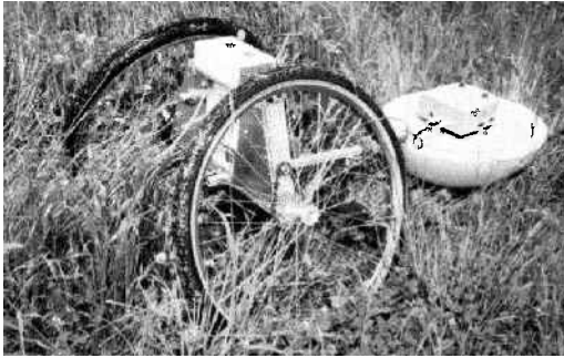
Figure 18.2 The robot Pemex. It is a prototype for a demining robot, built at the LAMI-EPFL in Lausanne, Switzerland (reprinted with permission).
