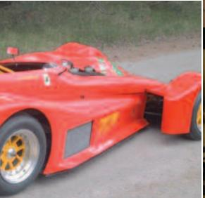
in 2002. Differing from the UK-built version, which was last updated in 1994, the chassis featured improvements to the lower front frame as well as a redesigned nose frame and front suspension rocker arms. In addition, the chassis was bolted directly to the back of the engine, making it more of a structural member.
