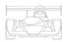
LEFT The S240, offered up here in 2D CAD form, could take the Clubmans-type cars in a different direction. The lefthand-drive configuration was dictated by the positioning of the exhaust ports to the right of the Honda engine
