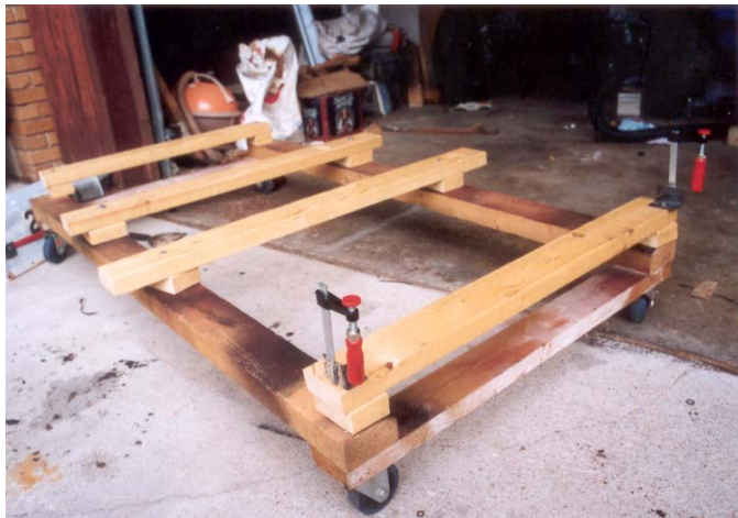
This cart will hold the body tub for painting and body work. Note the adjustable lifts for the rear shelf.
