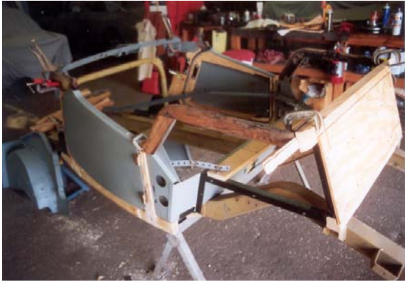
The doors are hung, but without sheet metal, the body tub looks pretty insubstantial.
