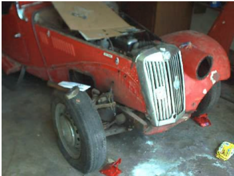
The TF project is finally underway: The fenders come off ... Soon the body tub will be lifted off the frame and painting begins
