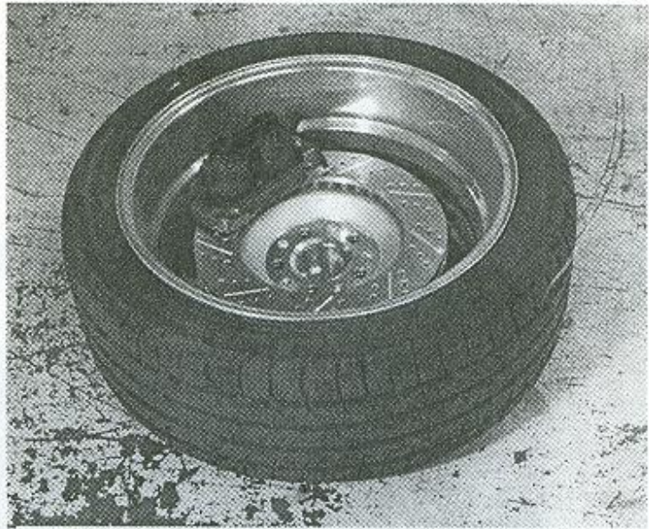
Place brake assembly in wheel and rotate to ensure proper clearance.
