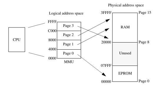
Each MMU register represents one logical page and contains a mapping to the corresponding physical page. Example: the picture above shows one possible mapping where logical page 0 is mapped to physical page 0, logical page 1 is mapped to physical page 10 etc. In table form it looks like this:
