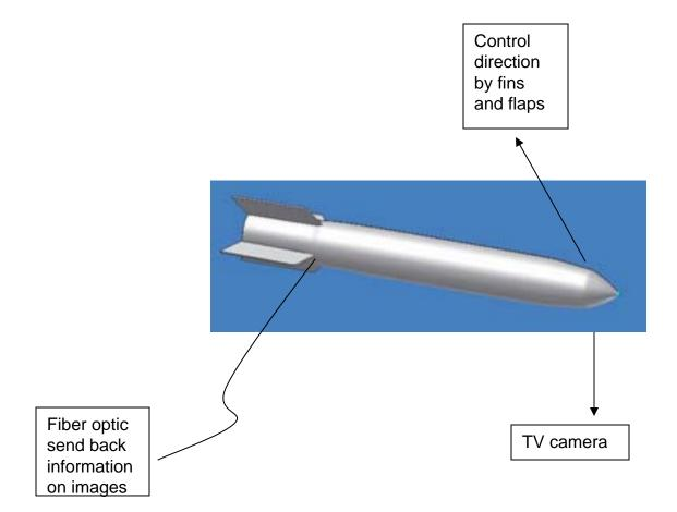
Missile guidance system using TV camera (real time image)
