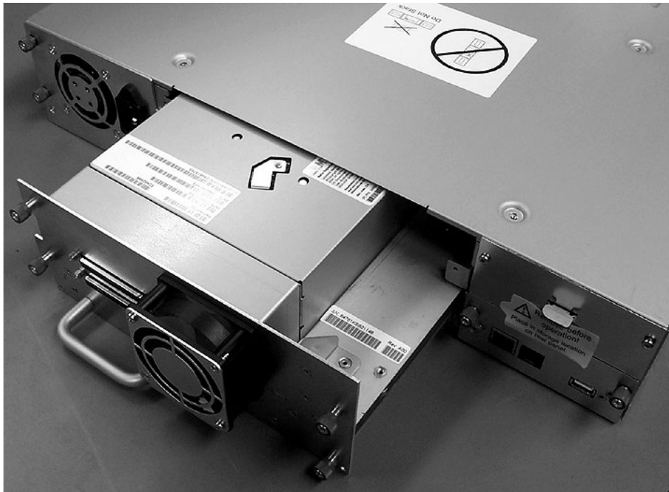
Figure 6. Install tape drive
