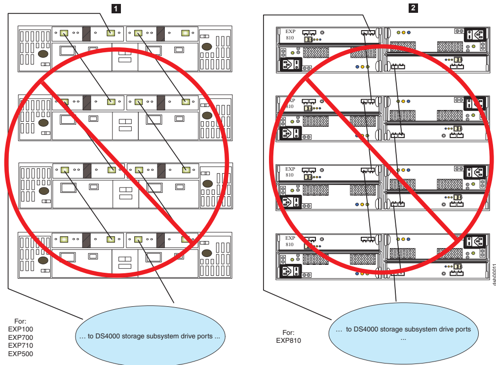
Figure 13. Not recommended alternate cable loop scheme for when connecting DS4000 storage devices
