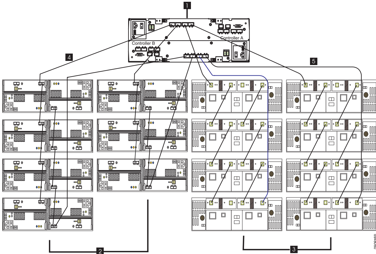
Figure 5. DS4800 configuration with 2-Gbps and 4-Gbps enclosures in different drive channel pairs
