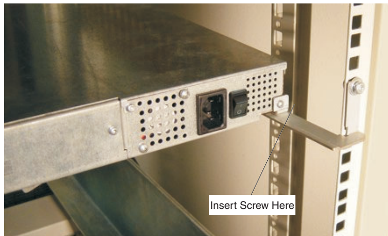
Figure 11. Attaching the autoloader to the rails
