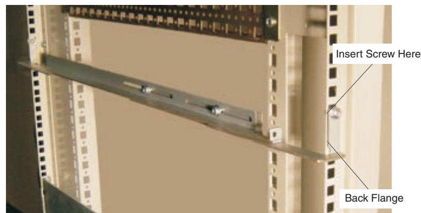
Figure 9. Attaching the left side rail to the back of the rack
