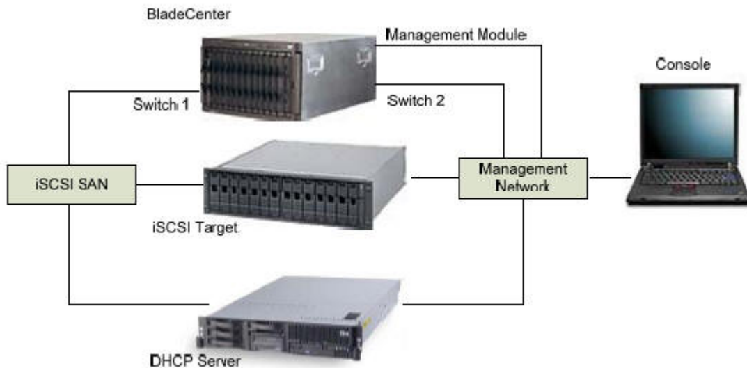
Figure 2. SAN with DHCP configuration
