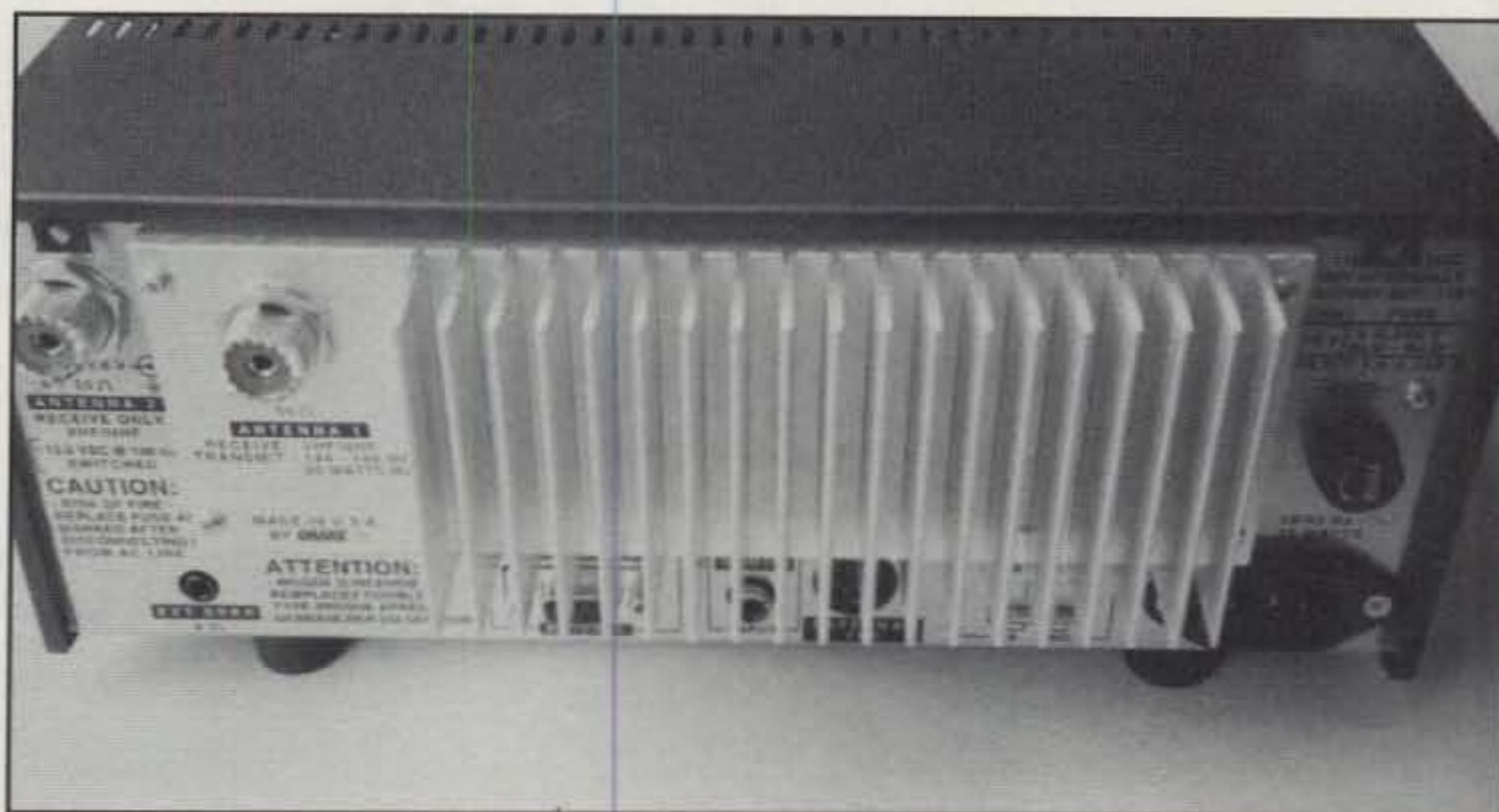
Rear view of the TR270 reveals massive heatsink, dual antenna sockets, and ports for computer interfaces.
