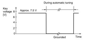
If the key voltage is more than 8 V, switch the mode switch (S1) to OFF mode (lower position).
