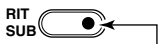
Lights red while the RIT function is activated; green while the SUB DIAL function is activated.
