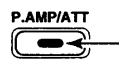
Lights green while the preamp is activated; lights red while the attenuator is activated.
