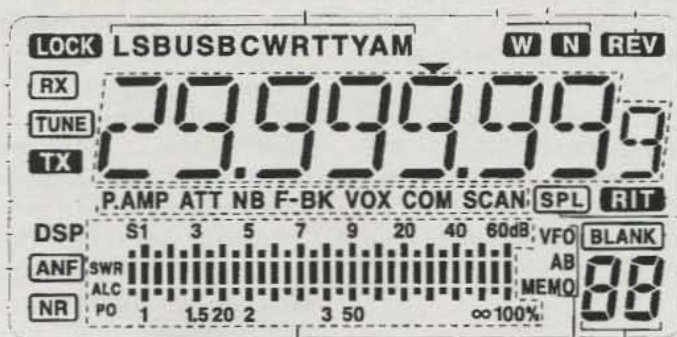
Fig. 2— A “show all” analysis of the IC-718’s front-screen display. The screen shows selected frequencies, memories, and all operating parameters, plus a multi-function bar-graph-type meter.
