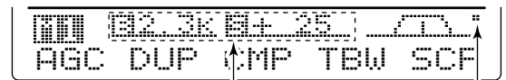
Passband width and shifting value are indicated while [TWIN PBT] is operated. Appears when PBT is used.
