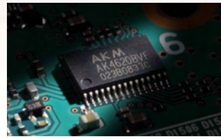
<AD/DA converter> AK4620B ADC Signal/(Noise+Distortion) : 100dB ADC Dynamic range, S/N : 113dB DAC Signal/(Noise+Distortion) : 97dB DAC Dynamic range, S/N : 115dB
