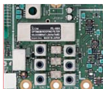
1.2kHz Optimum Roofing Filter 3, 6, 15kHz High-Spec 1st IF filters
