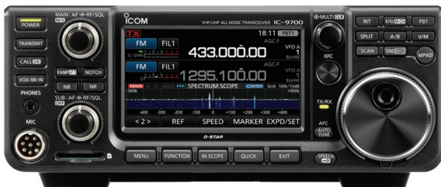
The front panel of the IC-9700 tri-band transceiver - 2m, 70cm and 23cm.
