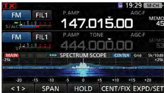
Figure 1 — The Icom IC-9700's expanded spectrum scope with waterfall.
