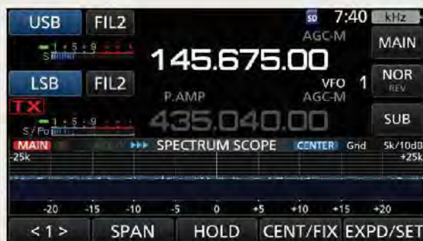
Figure B — The IC-9700 setup for Mode B satellite operation.
