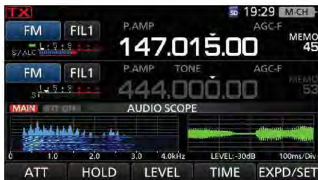
Figure 2 — The Icom IC-9700's audio scope.
