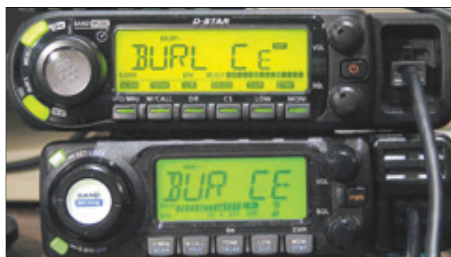
Figure 1 — Compare the ID-880H display with the older ID-800H below. The '880H is wider, a bit more cluttered, but still easy to read. The '880H display can show eight characters compared to the ID-800H's six. The ID-880H has one extra button, but the button labels are printed on the panel and disappear in the dark. The bottom row of icons shows the button's secondary (push and hold) functions.
