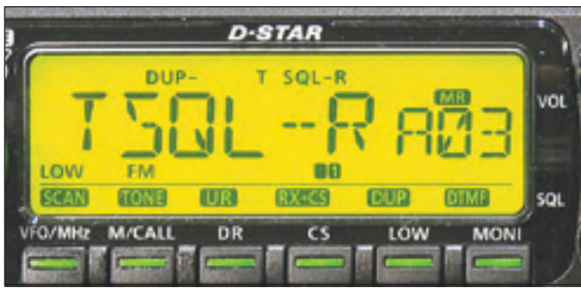
Figure 2 — Selecting a tone mode in the ID-880H. The tone options shows up as big characters, not just tiny icons. This is the new reverse tone squelch mode described in the text.
