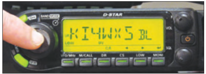
Figure 3 — Here I'm programming the ID-880H. Note the little arrows at the bottom of the display that aid navigation. Also note that the display shows eight characters (with the last two shrunk a bit). This call sign: KI4WXSBL is DPlus shorthand that says "link to the KI4WXS UHF repeater."
