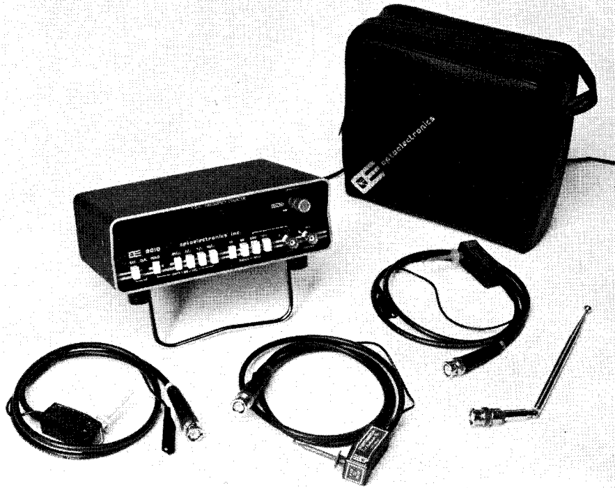
The Optoelectronics 8010 frequency counter and accessories. The probes, antenna and carrying case are optional. A wall transformer is supplied with the counter for ac operation.
