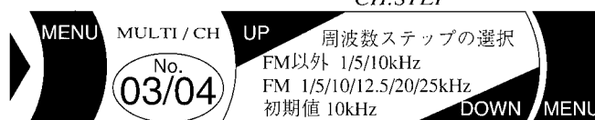
MULTI/CH control Frequency step size for SSB, CW, FSK, or AM mode MULTI/CH control Frequency step size for FM mode
