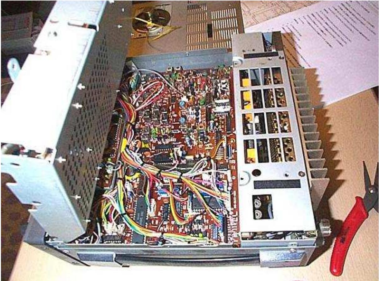
3. Take off the Control Unit by removing eight screws. No need to remove nylon connectors.
