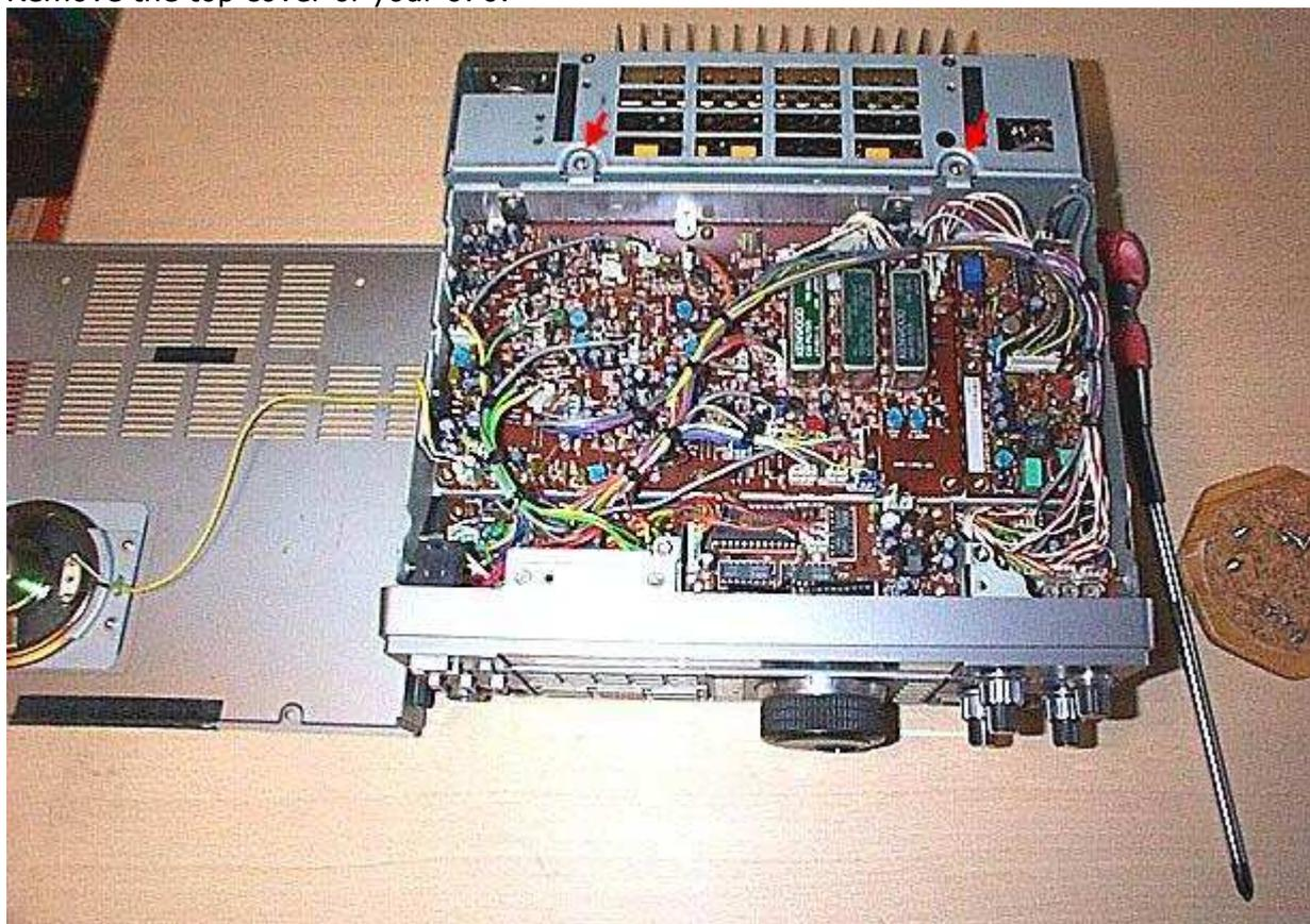
2. Lift the IF Unit by removing the two screws (shown with red arrow in the above picture).
