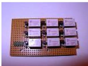
I didn t make a PC board layout for this prototype yet. Components were soldered on a perforated construction board (size abt. 8.5cm x 5cm). The board was mounted under the removable top cover with 3 screws. This space is reserved for the optional VS-2 Voice Synthesizer which I don t use.
