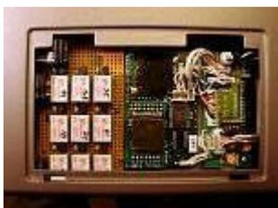
Now you can drive any remote antenna switch with the relay outputs from this band decoder.
