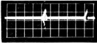
d. 100-KC SPECTRUM INPUT 1A2A2E10 0.2 VOLTS/CM 2 MICROSECONDS/CM
