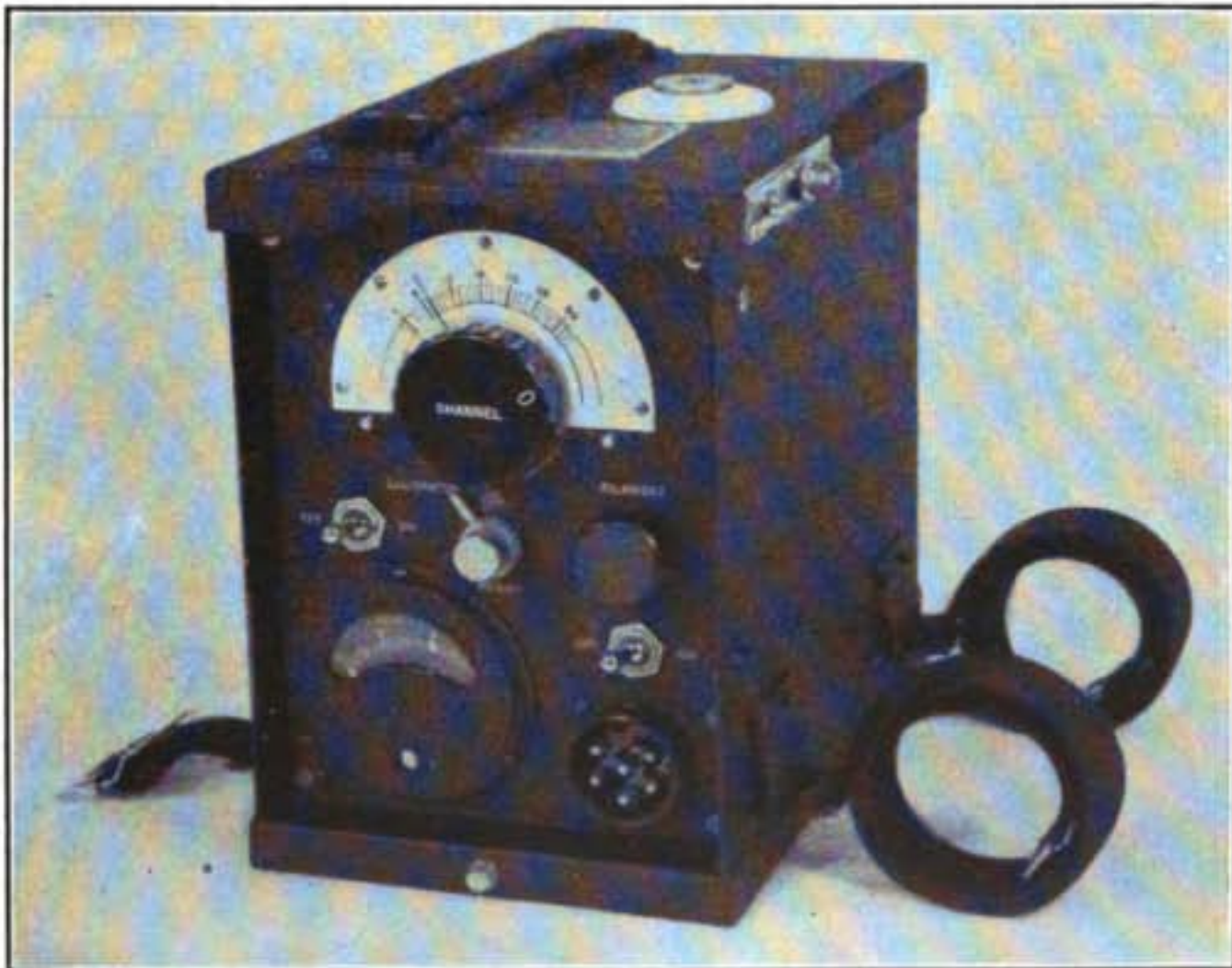
FIGURE 9.—Radio receiver and transmitter BC-322, front cover removed.
