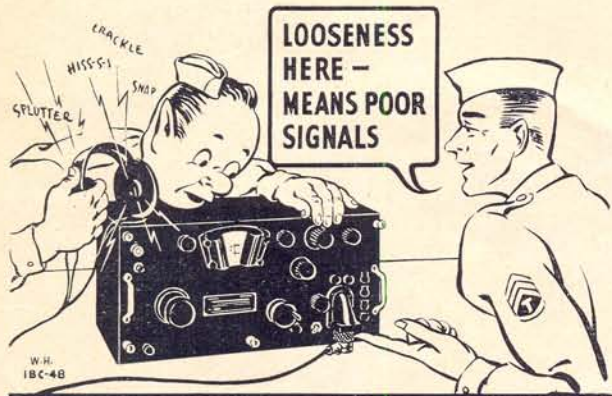
INSERT PLUGS OF THE PL-114 TYPE FULLY BEFORE YOU TIGHTEN THE KNURLED RING
