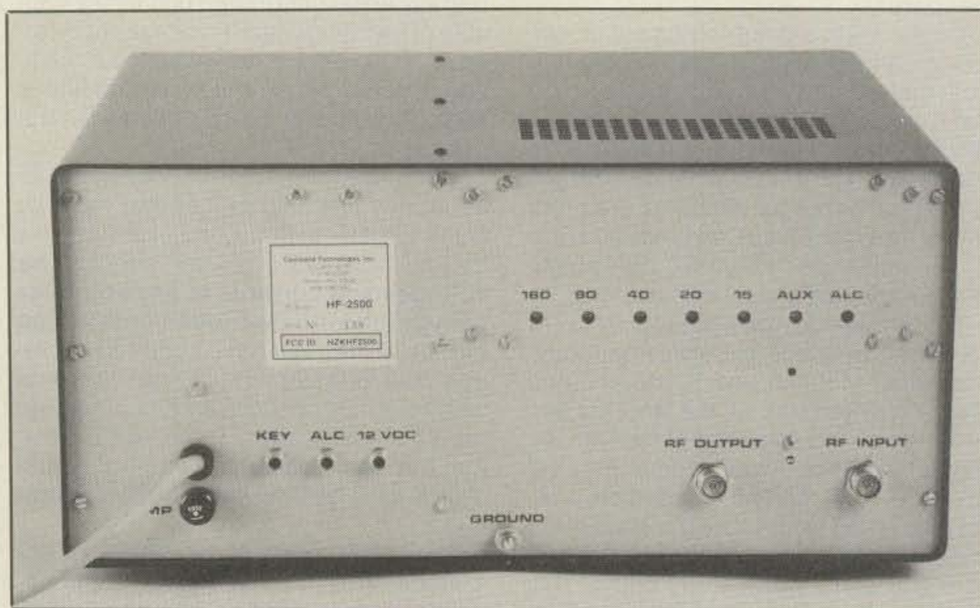
This is the rear view of the HF-2500. Along the upper right are the adjustment access holes for the input circuits and ALC adjustment. At the lower left are the KEY, ALC input, and an auxiliary 12 VDC output.
