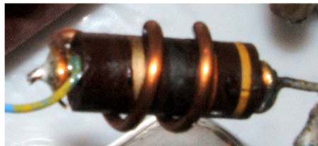
Figure 5.0 Parasitic Suppressor
