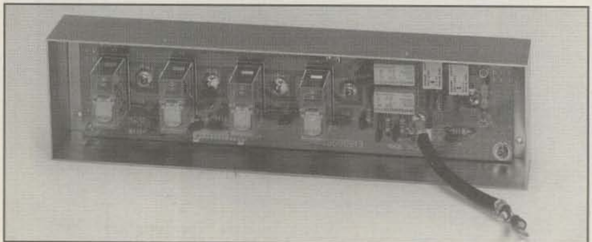
An interior view of the antenna switching network.
