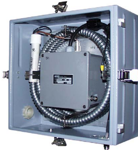
Fig. 9: Inside view of antenna box: Impedance adaptor and Transmission line
