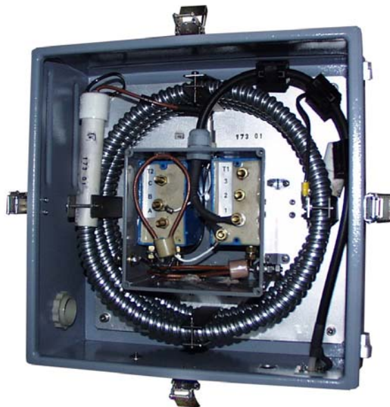
Fig. 10: Inside view of impedance adaptor: Broadband Transformers
