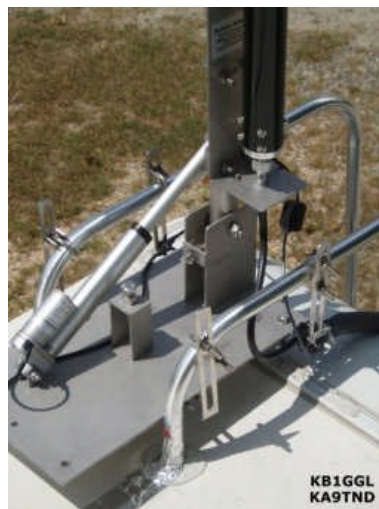
Picture 4 – MT-1 & Automatic Lift & Lay
