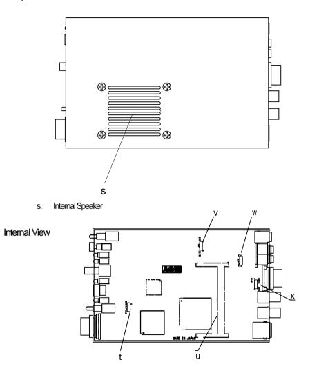
t. Factory setting jumper Must be set between 2-3. (Do not change this setting at any time.)
