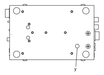
y. Microphone output level Refer to Level Adjustment Radio Input Level at page 18 for details
