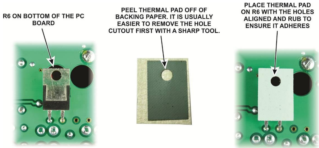
Figure 15. Placing Thermal Pad on R6.
