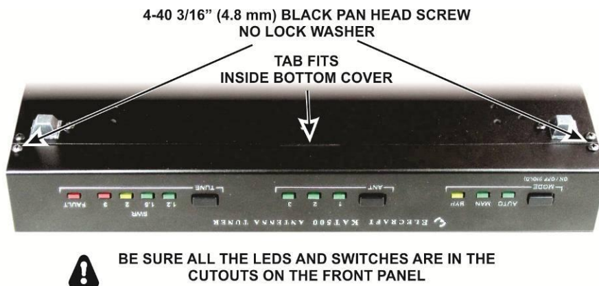
Figure 32. Mounting the Front Panel.
