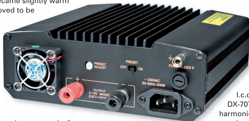
Fig. 3: The back of the unit has the main output terminals as well as two lesser used controls.
