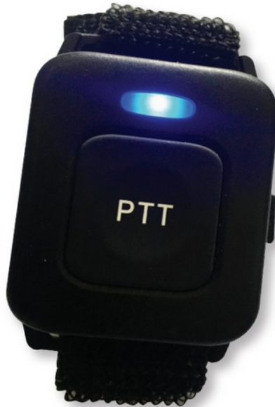
The AT-D878UV Plus is fitted with a Bluetooth module and comes with the Bluetooth PTT shown here.
