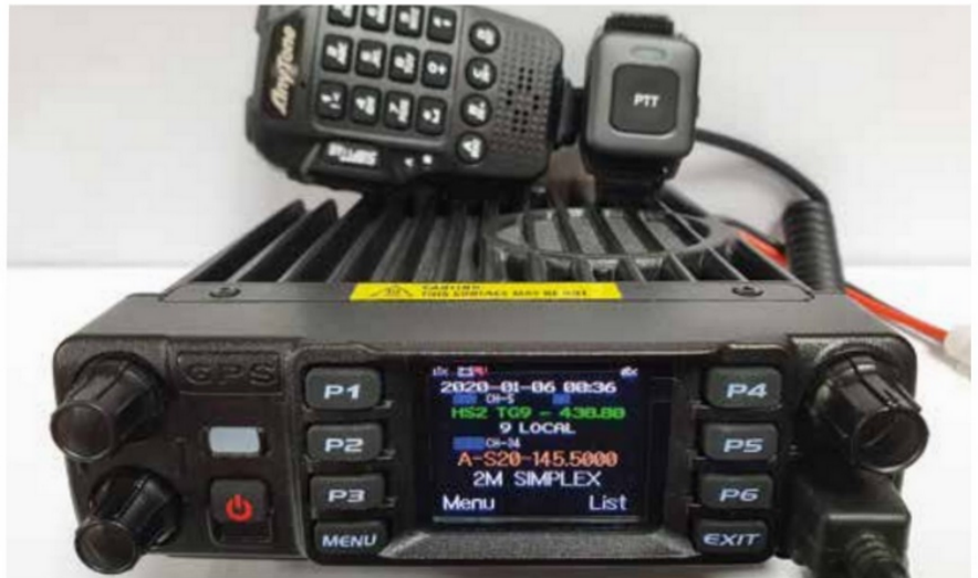
The Anytone AT-D578UVPRO is a dual band DMR/FM mobile transceiver.
