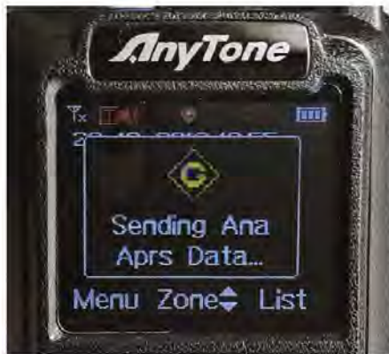
Figure 8 — The AnyTone AT-D878UV sending an APRS beacon.
