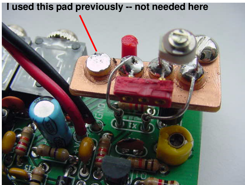
Figure 2. Note use of DIP pins at X1 used as a crystal socket. Also the 3-pin section of DIP pins used on the VXO Support.
