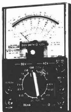
A TYPICAL MULTIMETER
